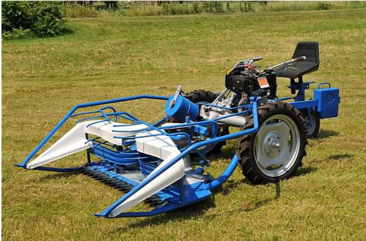
Picture 3. BCS 622 two-wheels tractor with STANDARD binder and operator's trolley
