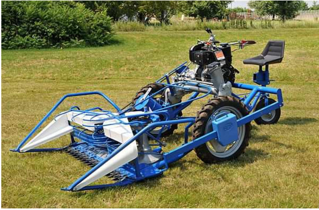
Picture 4. BCS 622 two-wheels tractor with SPECIAL binder and operator's trolley
